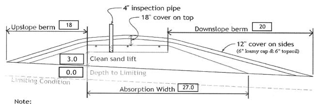
For 0 to 1% slopes, *Absorption Width* is measured from the *Bed* equally in both directions. For slopes >1%, *Absorption Width* is measured downhill from the upslope edge of the *Bed*.
