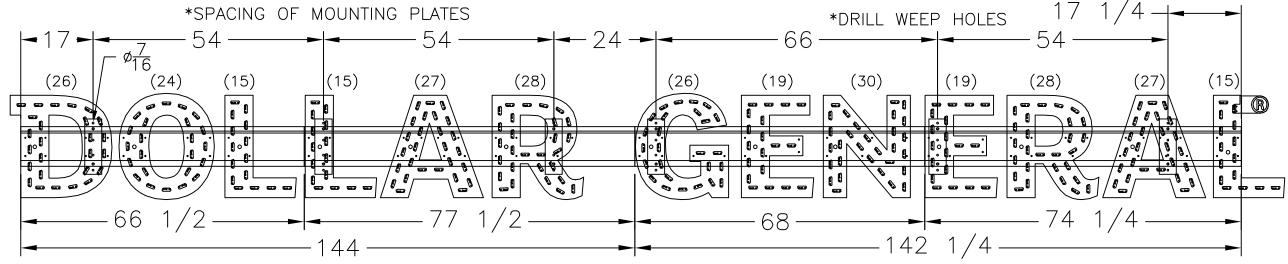
\*BOLT LETTERS TO RACEWAYS USING 1/4" HARDWARE
