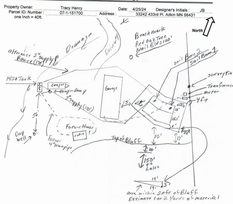
Top of Survey Pin NE of Power Transformer Elv.= 105.5'
