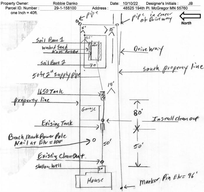
Existing tank inlet Elv.= 97.2' Estimated New 1650 tank inlet Elv.= 95.7' Grade at Power pole near House Elv.= 98.7' Nail on Power Pole near House Elv.= 100' Top of Super Pin at SW of House Elv.= 96' Grade at Pin Elv.= 95.1'
