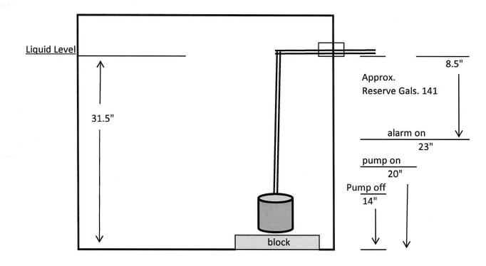
Assumes 10" pump Pump out dose at 5.6" = (85 gals. dose + 8 drain back) = 93 pump out gals.  $600 \text{ gpd} \div 7 = 85 \text{ gals.}$  Per Dose
