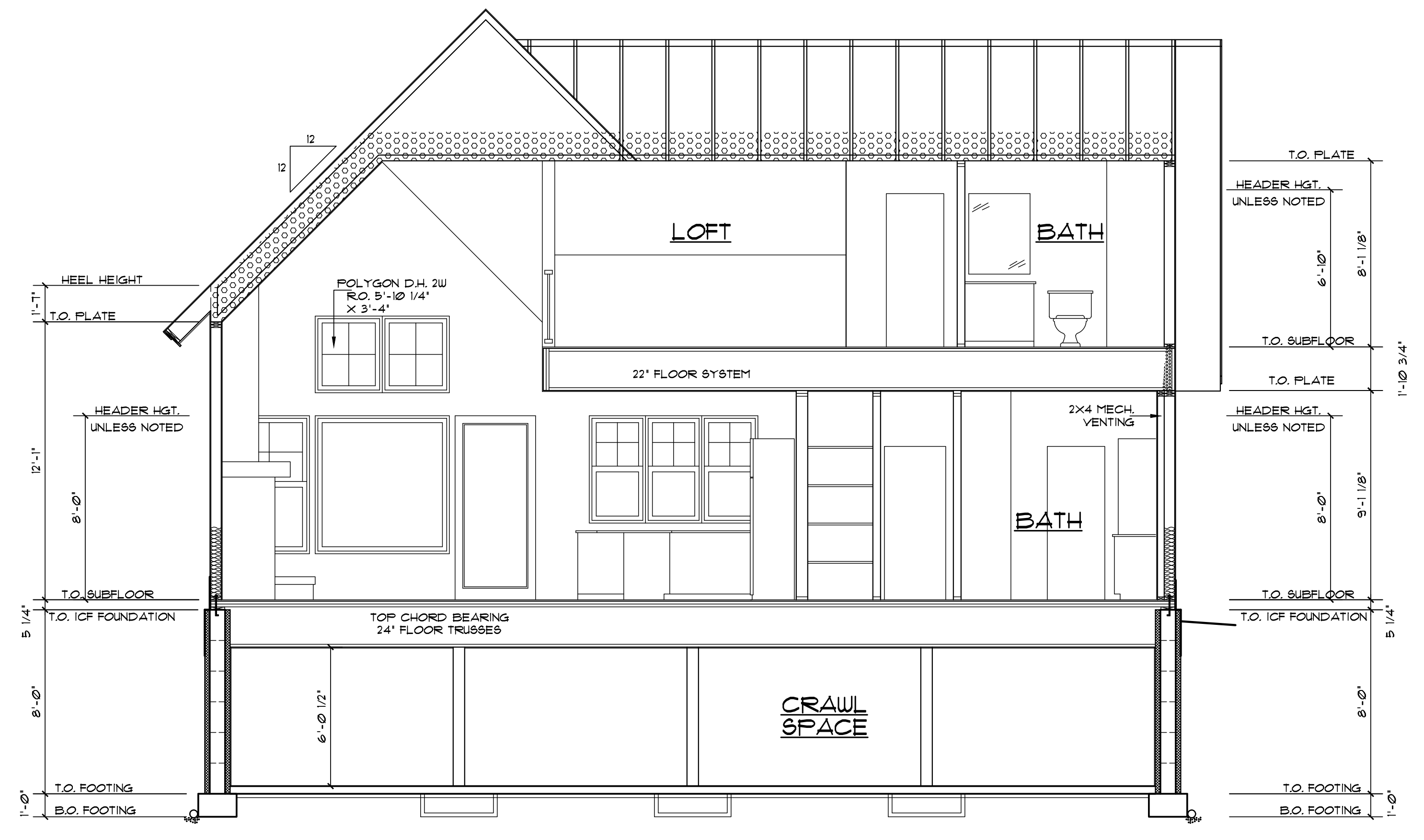
2 BUILDING SECTION SCALE: 1/4" = 1'-0"
