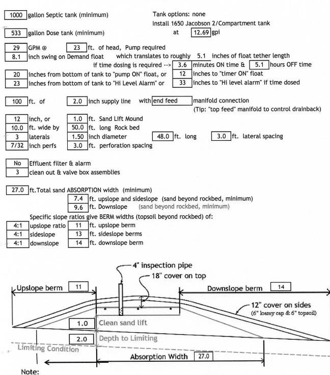
For 0 to 1% slopes, *Absorption Width* is measured from the *Bed* equally in both directions. For slopes >1%, *Absorption Width* is measured downhill from the upslope edge of the *Bed*.
