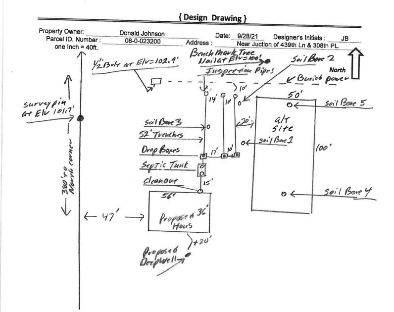
top of Survey Pin SW of Power Transformer Elv. = 101.7' 1/2 " bolt on South side of Power transformer Elv. = 102.9'
