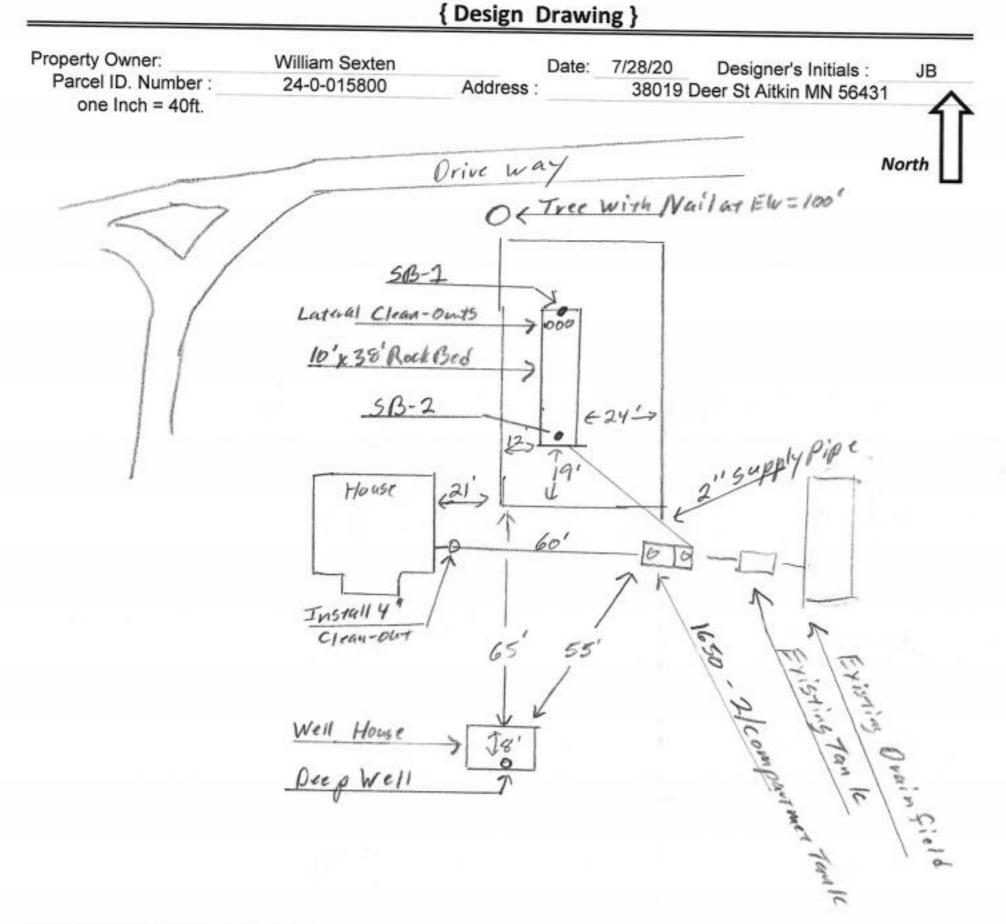
Existing Septic tank Inlet Elv.= 91.7' Grade at Existing Septic Tank Elv.= 92.4' Grade at New Tank Location Elv.= 95'
