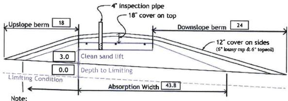
For 0 to 1% slopes, Absorption Width is measured from the Bed equally in both directions. For slopes >1%, Absorption Width is measured downhill from the upslope edge of the Bed.
