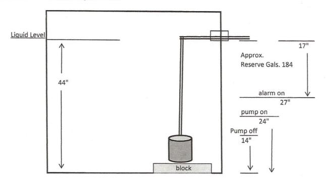
Assumes 10" pump Pump out dose at 9.8" = (75 gals. dose + 31 drain back) = 106 pump out gals.  $450 \text{ gpd} \div 6 = 75 \text{ gals.}$  Per Dose
