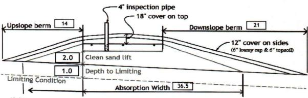
For 0 to 1% slopes, *Absorption Width* is measured from the *Bed* equally in both directions. For slopes >1%, *Absorption Width* is measured downhill from the upslope edge of the *Bed*.
