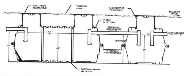
The IM-540 is an injection molded two piece mid-seam plastic tank. The injection molded plastic design allows for a mid-seam joint that has precise dimensions for accepting an engineered EPDM gasket. Infiltrator's gasket design utilizes technology from the water industry to deliver proven means of maintaining a watertight seal.
