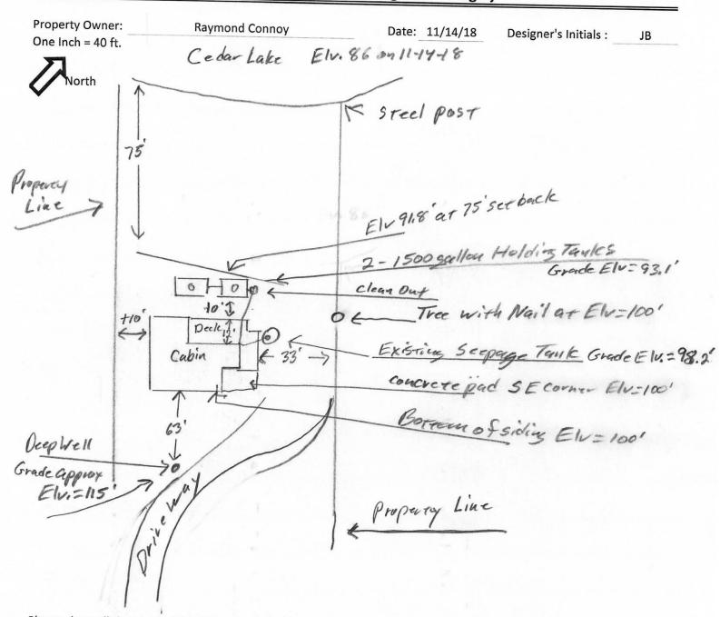
Please show all that apply (Existing or Proposed):Please Draw to Scale with North to Top or Left Side of Page:Wells within 100ft. Of Drain field.Disturbed/Compacted AreasAccess Route for Tank MaintenanceWater lines within 10 ft. of Drain field.Component LocationProperty LinesDrain field Areas:OHW ordinary high waterStructuresLot EasementsSetbacks
